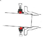
ONE-LOK's cam action also accommodates deflection of the joint during installation, and also allows for subsidence, seismic or other forces after installation, up to the maximum allowed deflection.
