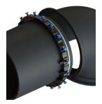
3. Insert the gasket along with the pipe into the fitting socket and seat the gasket firmly and evenly into the gasket cavity, keeping the joint straight.
