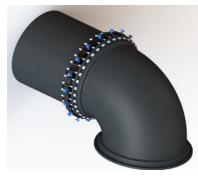
1. Clean the fitting socket & pipe end. Lubricate mechanical joint gasket & pipe end with soapy water or approved lubricant meeting AWWA C111/A21.11. (A transition gasket is required if using on steel OD pipe)
